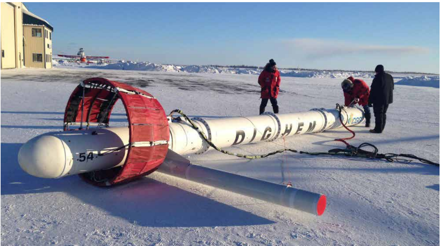
Configuring the Resolve6 AEM and magnetic equipment for a survey in winter conditions. (Northwest Territories). Photo credit: Xcalibur Multiphysics
