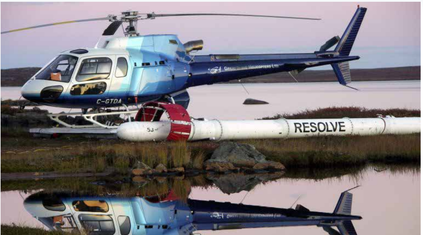
The Resolve6 AEM system and helicopter preparing for a survey in the Northwest Territories. Photo credit: Xcalibur Multiphysics
