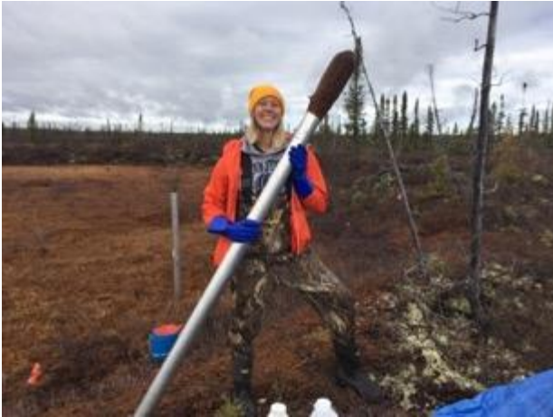
Figure 10. Frozen finger sampling in thermokarst bog features. McCuaig with frozen finger sampler (right) and a sample with water (frozen due to the sampling technique) between peat layers demonstrating the structure of these peatlands.
