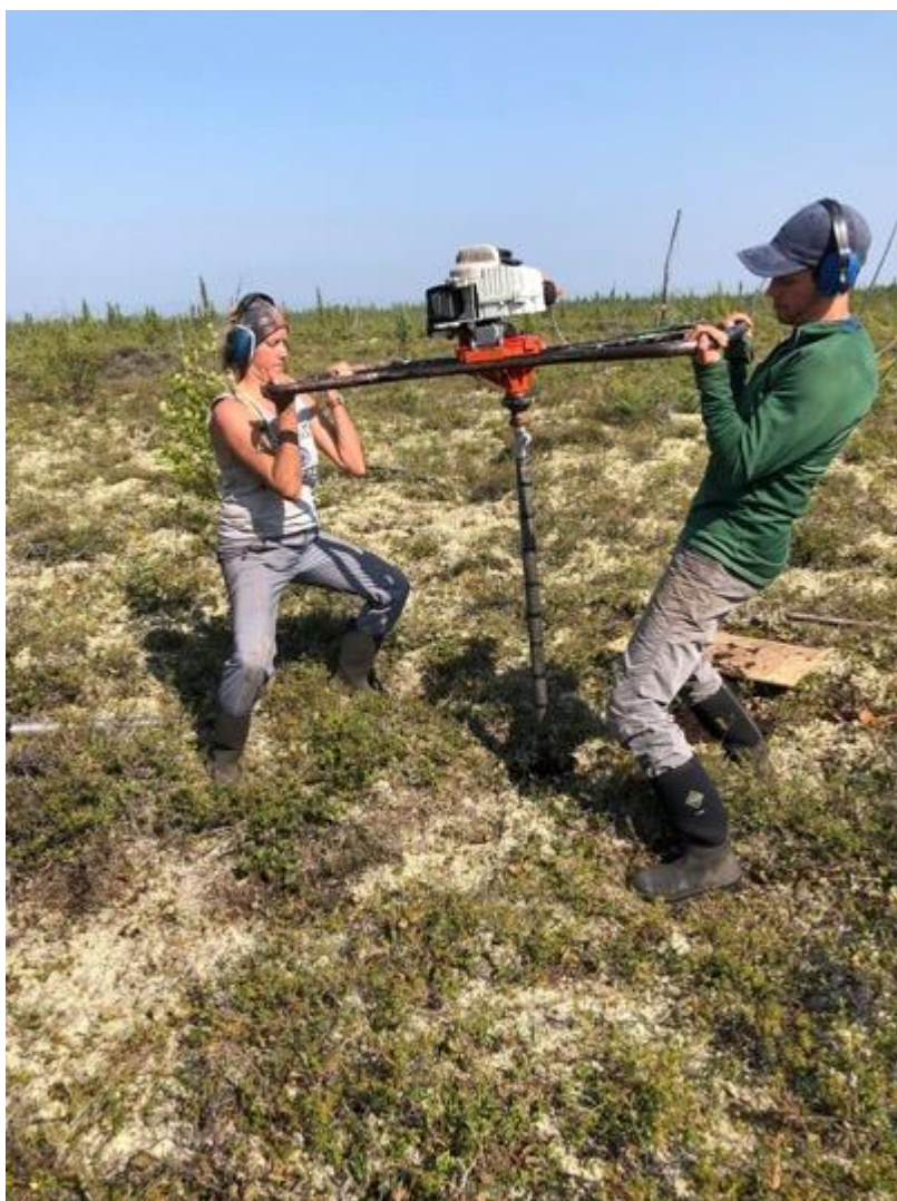
Figure 9. McCuaig and Paul coring permafrost in a lichen peatland (left) and peat-rich permafrost core segment (right).
