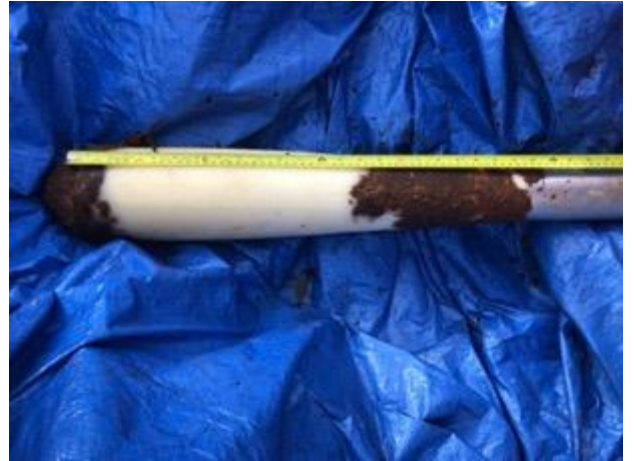
Figure 10. Frozen finger sampling in thermokarst bog features. McCuaig with frozen finger sampler (right) and a sample with water (frozen due to the sampling technique) between peat layers demonstrating the structure of these peatlands.
