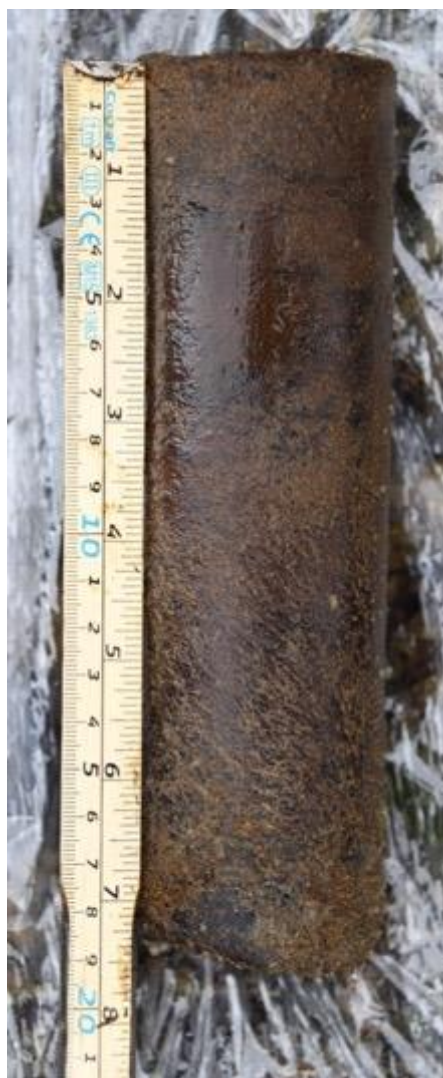
Figure 9. McCuaig and Paul coring permafrost in a lichen peatland (left) and peat-rich permafrost core segment (right).
