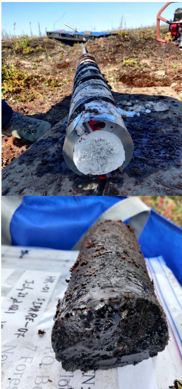
Figure 7. Two permafrost cores from permafrost monitoring sites. Top panel: a very ice-rich permafrost core. Bottom panel: a very carbon rich permafrost core.
