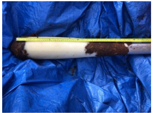
Figure 7. Frozen finger sampling in thermokarst bog features. McCuaig with frozen finger sampler (right) and a sample with water (frozen due to the sampling technique) between peat layers demonstrating the structure of these peatlands.
