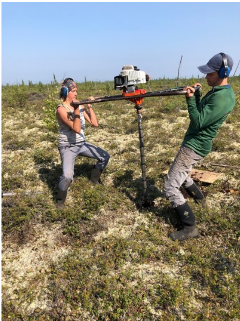
Figure 6. McCuaig and Paul coring permafrost in a lichen peatland (left) and peat-rich permafrost core segment (right).
