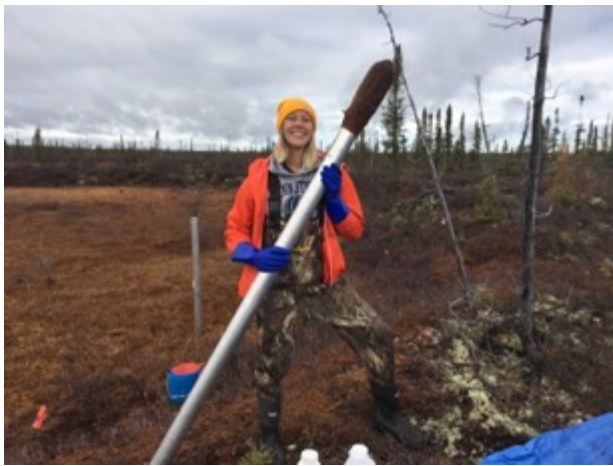
Figure 7. Frozen finger sampling in thermokarst bog features. McCuaig with frozen finger sampler (right) and a sample with water (frozen due to the sampling technique) between peat layers demonstrating the structure of these peatlands.
