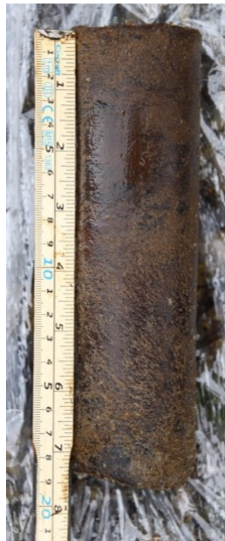
Figure 6. McCuaig and Paul coring permafrost in a lichen peatland (left) and peat-rich permafrost core segment (right).
