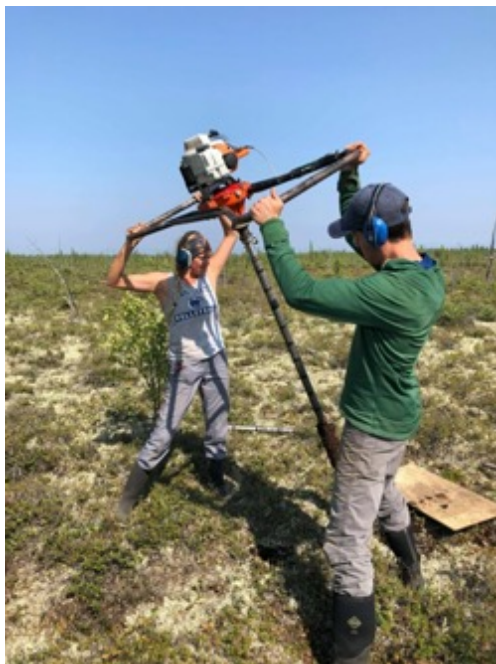
Figure 2. Permafrost coring and peat sampling in a collapse scar in the Sahtú region. Photos courtesy of Emily Ogden.
