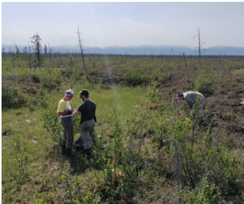
Figure 2. Permafrost coring and peat sampling in a collapse scar in the Sahtú region. Photos courtesy of Emily Ogden.
