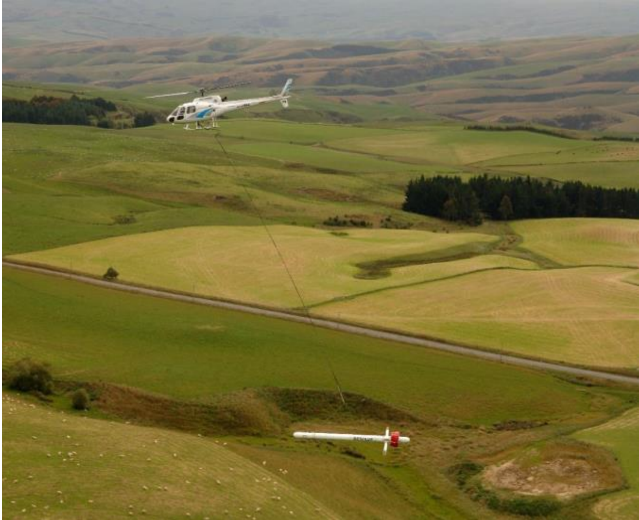
Figure 13. Resolve6 Airborne Electromagnetic system in flight. (Xcalibur Multiphysics, 2022).
