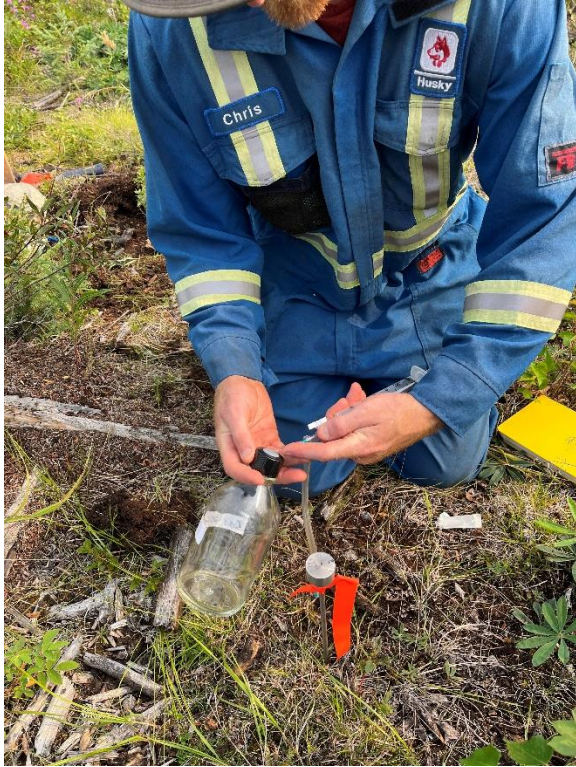
Figure 16. Shallow soil gas sampling with conventional soil gas probe.
