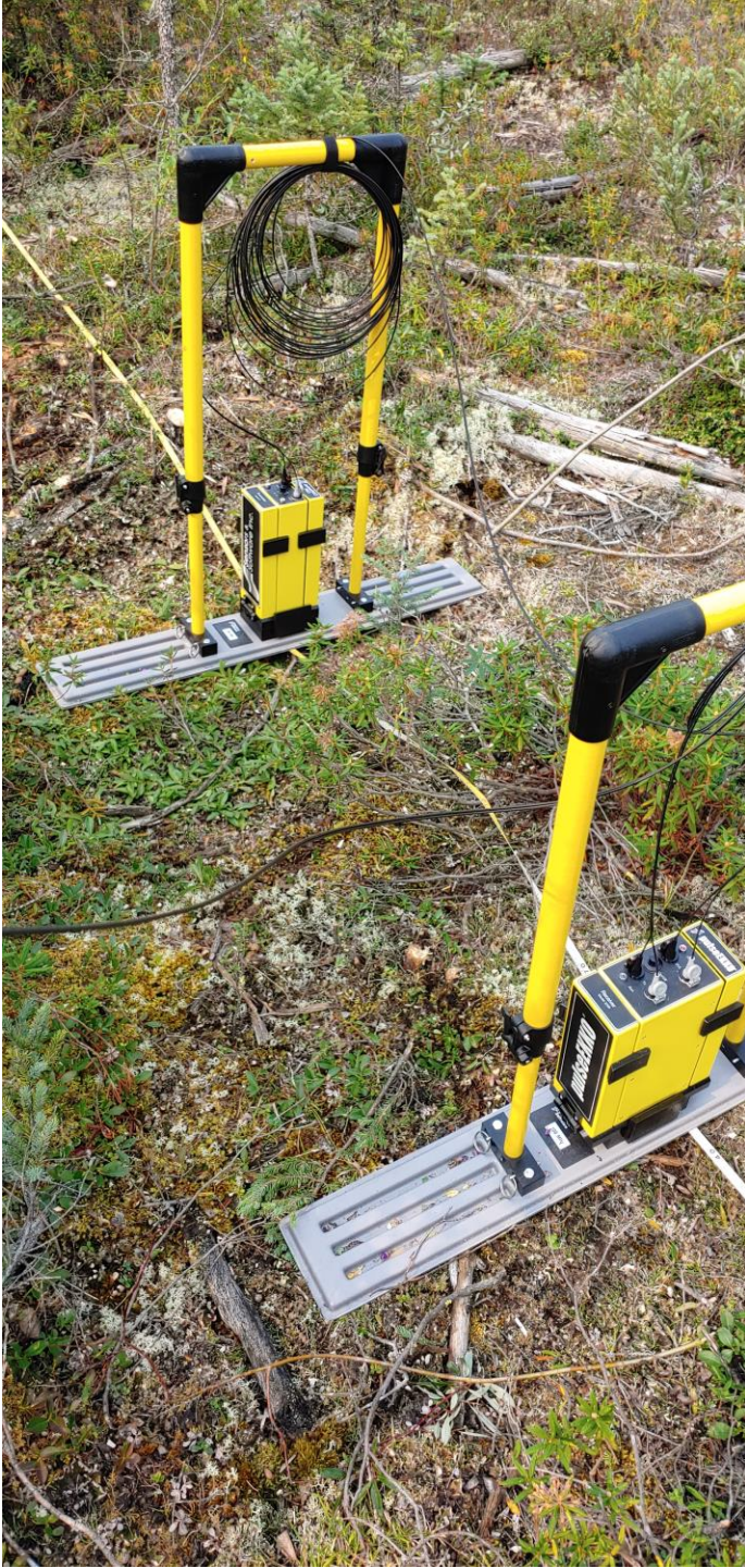
Figure 10. GPR equipment in the drill pad clearing at Site 1.
