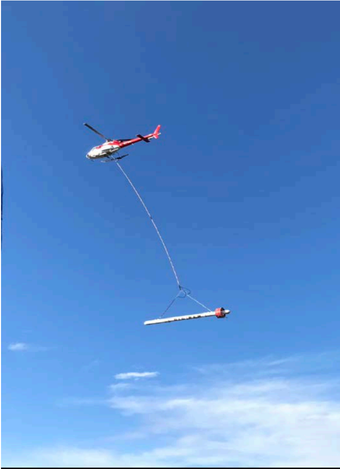
Figure 10. Resolve6 AEM system on site (a) and in operation (b). (Xcalibur Multiphysics, 2022).
