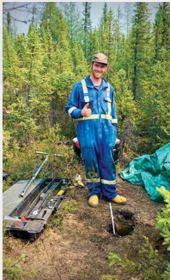
Coring of active zone and shallow permafrost within the Bogg Creek Watershed field site. Photo credit: Hugo Crites
