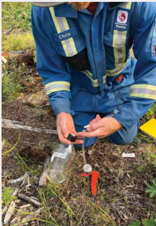
Soil gas sampling procedure with soil gas probe within the Bogg Creek Watershed field site. Photo credit: Hugo Crites
