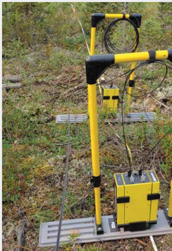
Ground penetrating radar across drill pad clearing within the Bogg Creek Watershed field site. Photo credit: Oliver Conway-White
